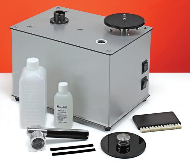
On top of the main unit you can see the pivot for the suction arm, the lower disc-clamp and the reservoir drain hole. Arranged around the base are the upper clamp, the arm (with spare velvet pads) and the brush that's used to spread diluted cleaning fluid over the record. The latter is prepared by mixing concentrate from the smaller bottle with tap water in the larger one - embossed with horizontal lines to help ensure correct proportions.
